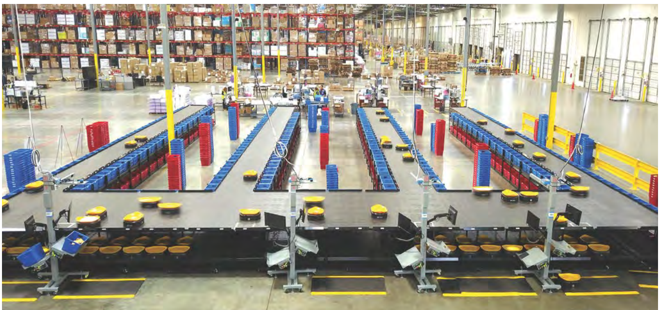
Tompkins Robotics’ t-Sort system employs free-moving, independent robots throughout the warehouse. Robotic automation such as this can improve logistics efficiency and transform supply chain visibility.
