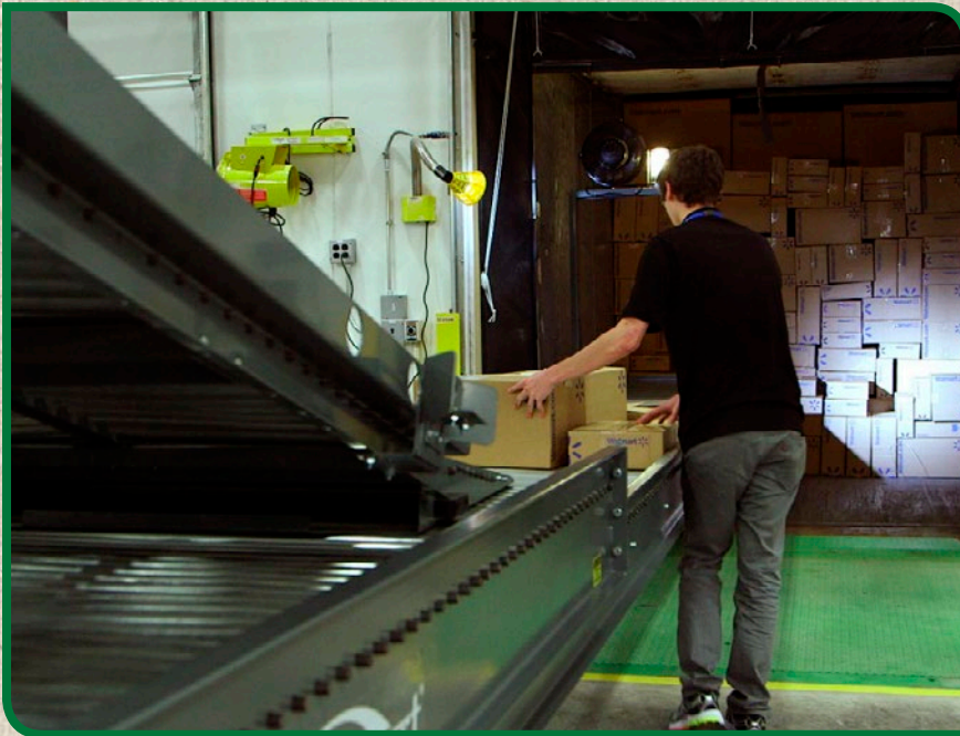
To conserve energy, Walmart moves products by conveyor rather than by forklift in its distribution centers.
