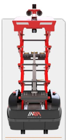
**inVia Picker:** Picking items as small as a pack of gum or as bulky as a case of soda, this robot provides a solution for e-commerce fulfillment centers through a Robots-as-a-Service platform. Pickers operate as an automated storage and retrieval solution, picking totes, bins, and boxes weighing less than 40 pounds from warehouse shelves. The robots can run on their own or work collaboratively with human operators.
