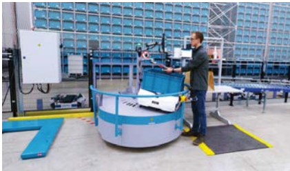
Sporting goods retailer Decathlon implemented Exotec's Skypod robotics system to improve order fulfillment processes and employee workstation ergonomics.
