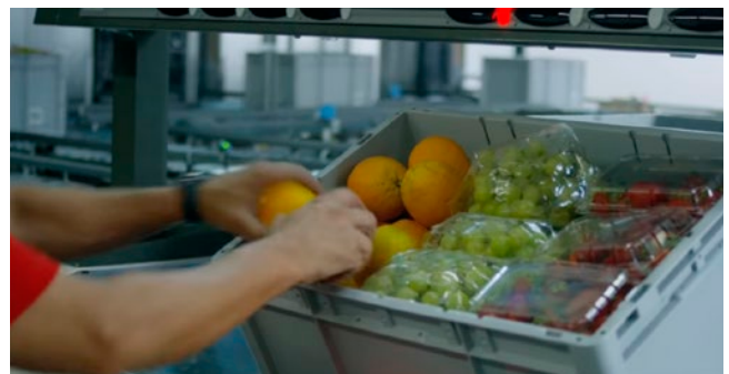
Albertsons Cos. partnered with Takeoff Technologies to fulfill e-commerce orders. The solution uses AI-enabled technology and a system of totes and conveyors to deliver items to Albertsons employees, who then prepare the order for the customer.
