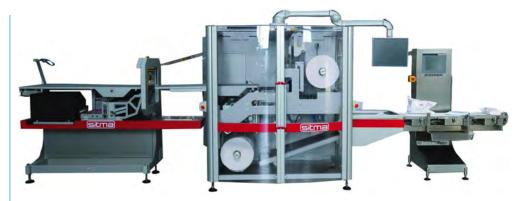
> Designed for e-commerce, **Sitma Machinery's** e-Wrap 2.0 can assemble packages and envelopes of varying sizes with different types of wrapping materials, including bio film and paper. The packaging machine can integrate a feeding system that prints and applies paper inserts, such as invoices, return notes, and other documents, to the packaging without glue.
