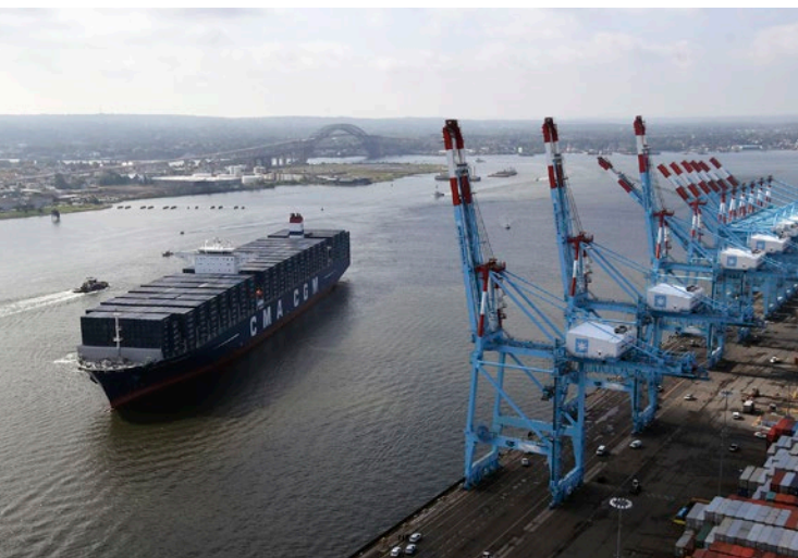
A post-Panamax containership docks at the Port of New York and New Jersey. The port invested in large-scale projects, such as the Harbor Deepening Program, so it could handle large vessels with capacities up to 18,000 TEUs.
