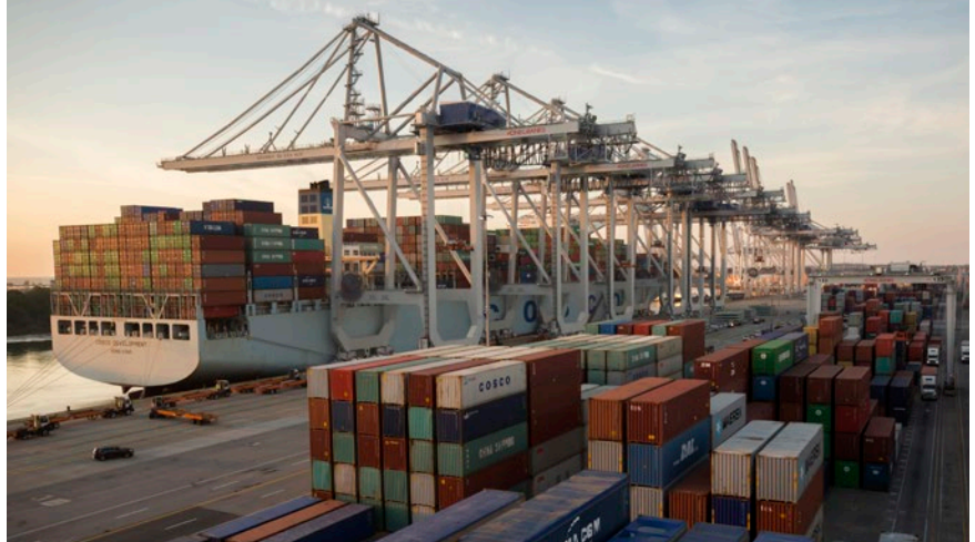
Georgia Ports Authority's new Panamax ship-to-shore cranes work the COSCO Development—the largest container ship ever to call on the U.S. East Coast—at the Port of Savannah.
