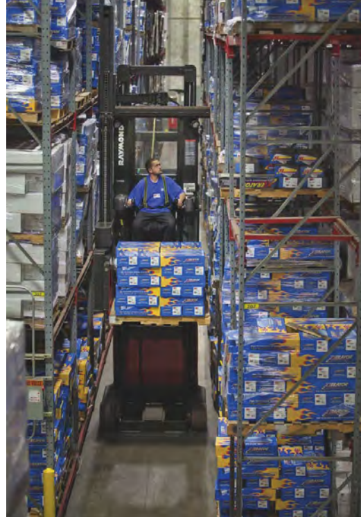
Intelligent technology directs a Raymond automated guided vehicle to move products between pickup and deposit points.
