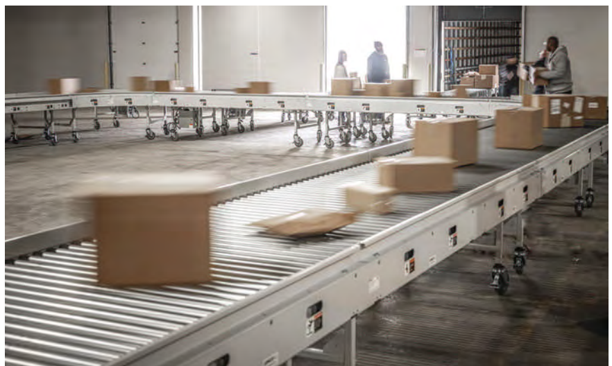
Modular portable roller conveyors from LogistiQ allow e-commerce centers to quickly install sorting capacity in smaller spaces than is possible with traditional conveyor systems.
