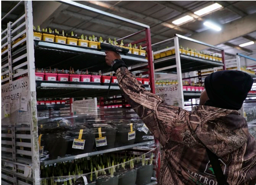
The Scan by Cart module uses data collected by RFID-powered handheld barcode readers to generate the shipping order information, documents, and labels Metrolina needs as it loads products onto trucks.
