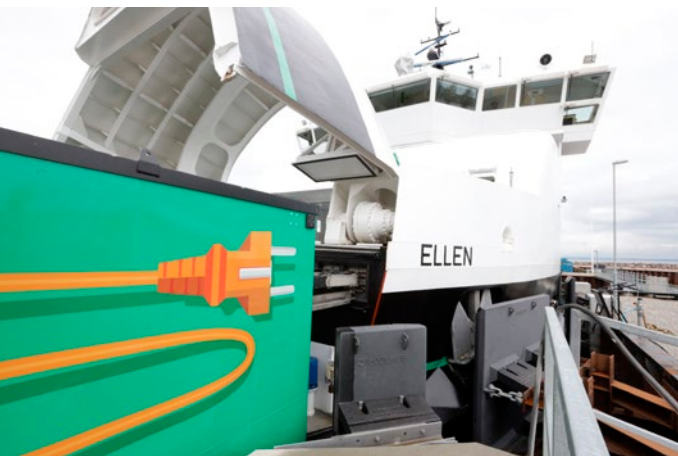
Among green initiatives in maritime logistics, the world's largest all-electric ferry, named Ellen , made its first commercial trip in August 2019. Capable of carrying about 30 vehicles and 200 passengers, the e-ferry is powered by a Leclanché battery system.
