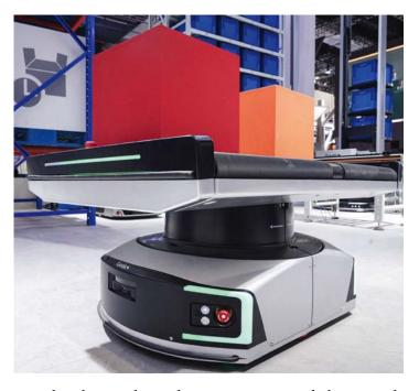
docking facilities. Equipped with an independent rotating control chassis and collision avoidance, the Sl00C can navigate narrow spaces.
