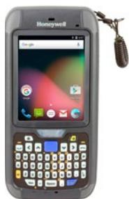
**Honeywell CN75 Mobile Computer:** This rugged handheld features smart battery technology that provides power for a full work shift, eliminating dead batteries and downtime. It's also equipped with a high-performance imager that scans barcodes accurately, even in low-light conditions, with motion tolerance to prevent delays. The powerful device features a 1.5-GHz dual-core, multi-engine processor with 2 GB RAM and 16 GB Flash.
