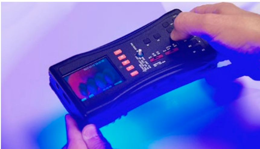
The FDA screens for counterfeit and sub-standard drugs with CD-3, a small, portable device that uses wavelengths of light to reveal differences between authentic and counterfeit drugs that look the same to the naked eye.
