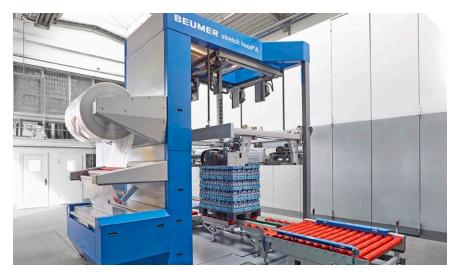
Conveying systems maker **BEUMER Group** unveiled its new stretch hood high-capacity system. The machine series offers higher throughput, and gentle transport of the film in the system. It also requires 40-percent less floor space than older systems. In addition, its opening hood lets workers in retail stores and logistics centers quickly remove the film when unpacking or repacking the goods, without using any cutting tools.
