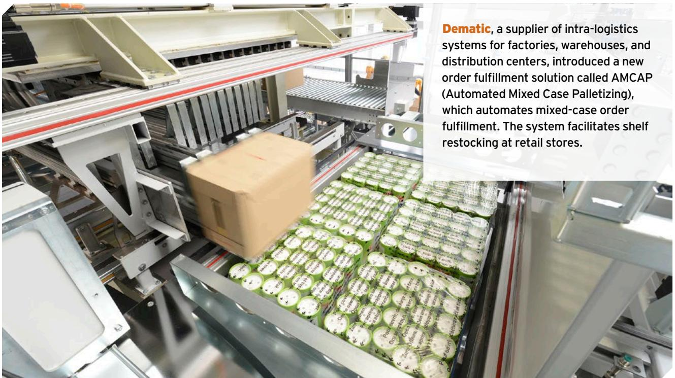
**Dematic**, a supplier of intra-logistics systems for factories, warehouses, and distribution centers, introduced a new order fulfillment solution called **AMCAP** (Automated Mixed Case Palletizing), which automates mixed-case order fulfillment. The system facilitates shelf restocking at retail stores.
