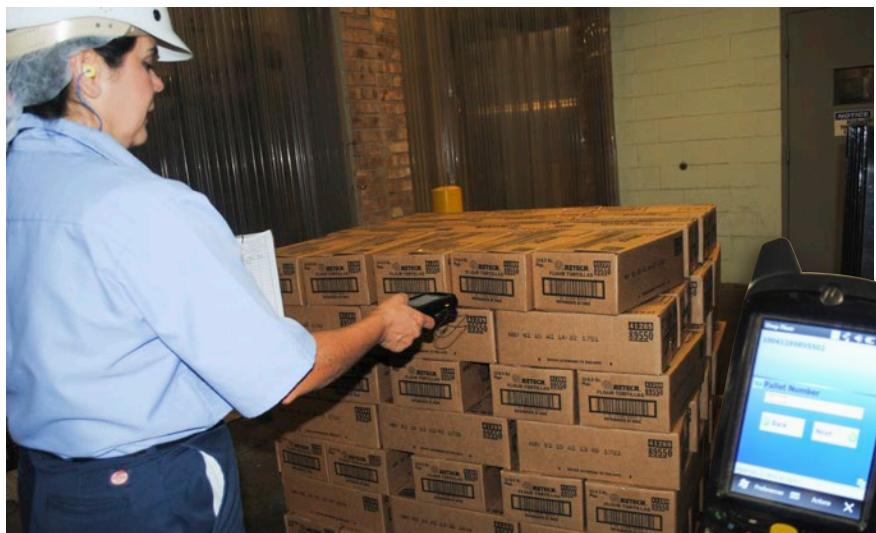
**A new barcode scanning solution provides Azteca Foods with full traceability of products moving into its finished goods warehouse.**
