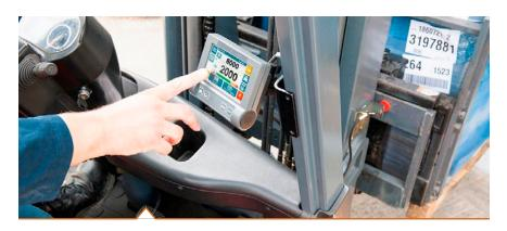
**Keytroller**, a manufacturer of electronic safety devices, introduced the PRECISE Hi-Accuracy Forklift Scale for forklift weighing. The hydraulic scale is nearly as accurate as carriage or fork load cell scales, achieving 0.2 percent maximum deviation at a lower cost. Equipped with a 4.3-inch color LCD touchscreen, the scale is water resistant and designed to withstand tough applications.
