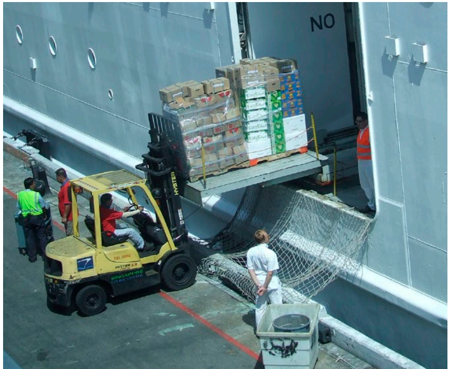
Workers use a forklift to load supplies onto a cruise ship while it’s docked at a turn-around port. Merchandise is stored on steel pallets for sanitation reasons.
