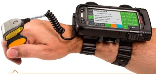
Honeywell Scanning and Mobility released a hands-free, wrist-mounted version of its Dolphin 70e Black mobile device. The device can be worn for extended periods of time, and features a large screen, flexible touchscreen keypads, and support for multiple scanner types.
