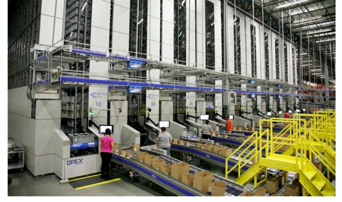
In goods-to-person order fulfillment, product moves directly to the operator, who can then pick what is needed to fulfill orders. This system increases the efficiency and accuracy of the picking process.
