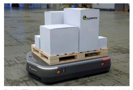
Clearpath's OTTO is a self-driving vehicle that effortlessly moves large items and standard pallets around a warehouse or distribution center.
