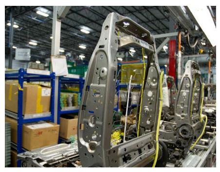
Carton flow racks, such as those used in Johnson Controls' 125,000-square-foot plant in Suwanee, Ga. - where seats, door panels, and other interior parts are assembled for the Kia Sorento - help create flexible, modular, and portable storage.
