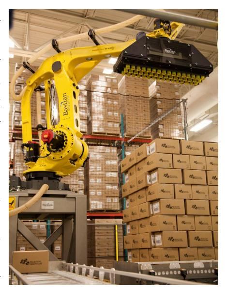
Bastian's palletizing robots can handle pallets, slip sheets, and tier sheets for completely automatic pallet building and depalletizing operations.
