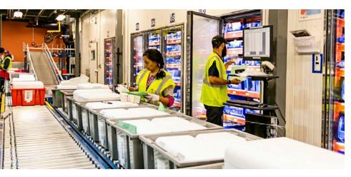
Pickers in Thermo Fisher Scientific's cold chain warehouse in Fredericksburg, Md., now fill orders in ambient temperature spaces. Deli-door style cases housing refrigerated products are on the first level; similar freezer cases are accessed via a second-level mezzanine.
