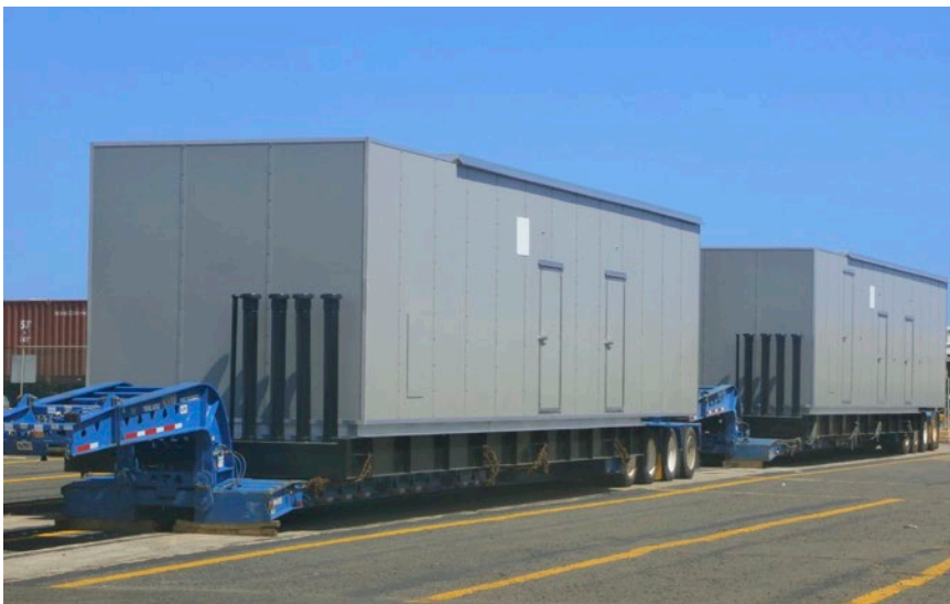
ATS International contracted Crowley’s liner services group to transport two 12-foot wide, 16-foot tall, 63-foot long enclosures containing generating equipment.
