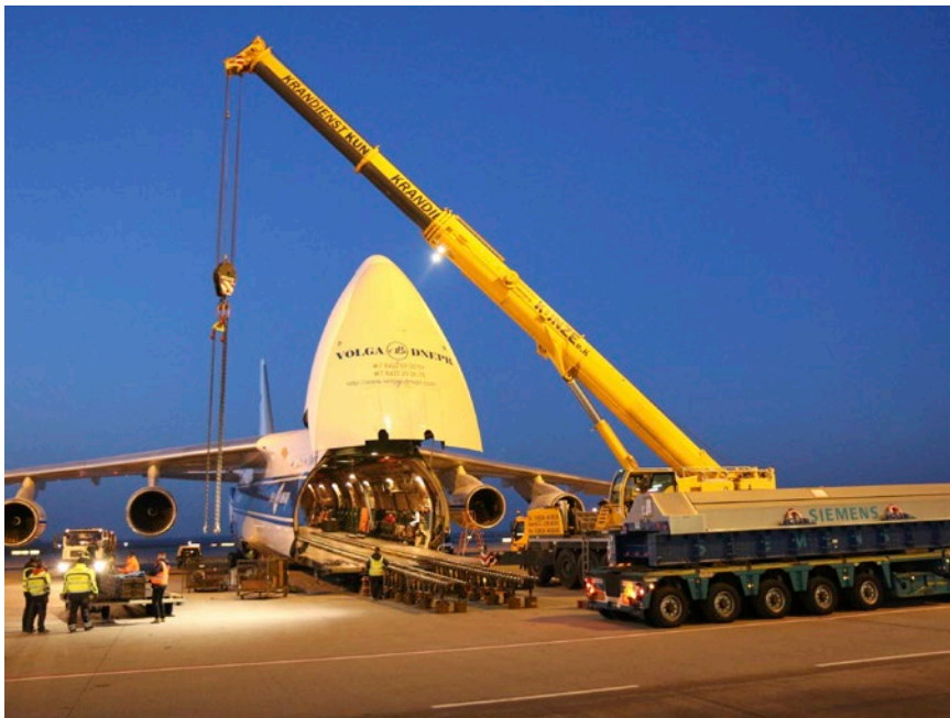
Siemens tapped the expertise of Volga-Dnepr Group’s Engineering & Logistics Centre to move a 50-ton rotor to Mumbai, India, onboard an An-124-100 freighter.
