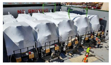
Railserve individually shrink-wrapped its locomotives to protect their exteriors from undue damage during transportation.
