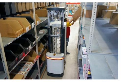
TORU Cube is able to grasp any size and weight rectangular object, store it in its built-in shelf, and deliver it directly to a shipping station.
