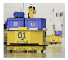
ADAM, Cimcorp's autonomous mobile robot, performs origin-to-random destination transportation of materials in Lean manufacturing operations.
