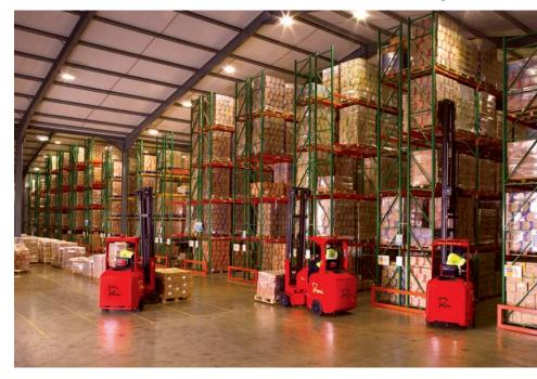
Narrow Aisle offers Flexi forklifts, which enable warehouses to store more inventory in less space. The VNA forklift can work in aisles as narrow as 6 feet 7 inches, while handling standard 48-inch-deep pallets.
