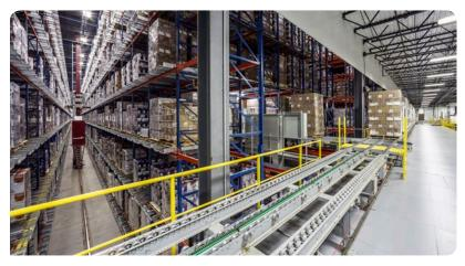
▲ The Glenmore Distillery opened a new distribution center featuring warehouse automation technology from Westfalia Technologies, a provider of logistics solutions for plants, warehouses, and distribution centers. The 223,000-square-foot facility in Owensboro, Ky., uses Westfalia's automated storage and retrieval system and the Savanna.NET warehouse execution system to store, retrieve, and manage pallets of finished goods.
