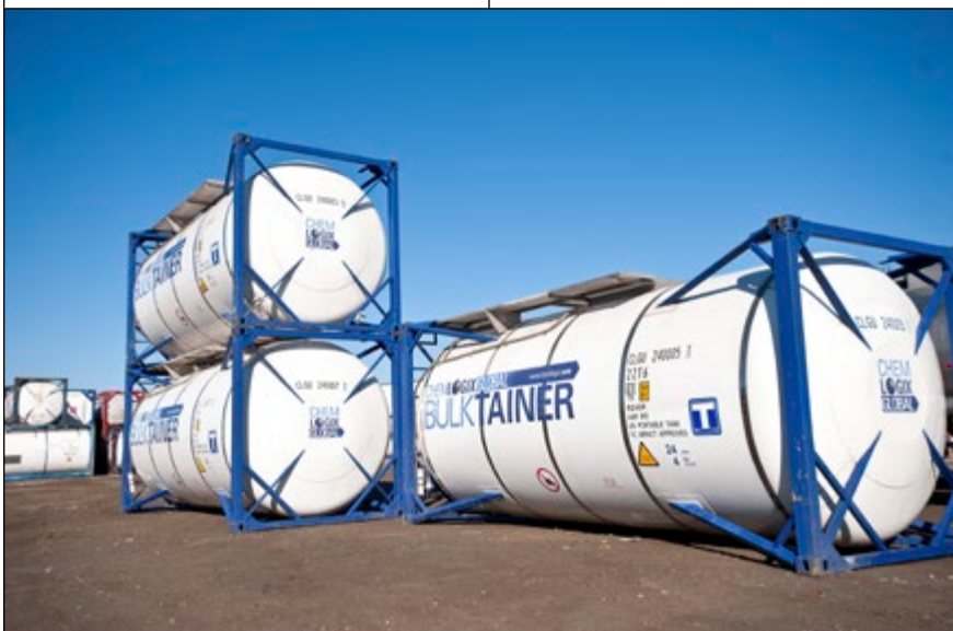
A division of CLX Logistics, ChemLogix’s intermodal service specializes in using bulk ISO intermodal tank containers to ship bulk liquid chemicals long distances.
