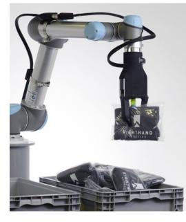
RightHand Robotics introduced RightPick, a combined hardware and software solution that can pick individual items to support e-commerce order fulfillment. Unlike traditional factory robots, RightPick handles thousands of different items using a machine learning backend coupled with a sensorized robot hand that works with all industry-leading robotic arms.
