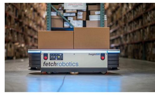
Fetch Robotics introduced two autonomous mobile robots to its fleet: Freight500 and Freight1500. Both new robots automate the delivery of bulky and heavy loads. Freight500 can move substantial loads, yet still fits through doorways and areas that people commonly traverse. For even bigger hauls, Freight1500 can support up to 3,300 pounds. Freight1500 can move standard-sized pallets as well as much bulkier cargo.
